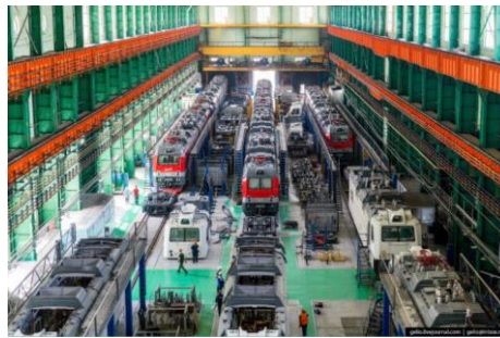
Picture 1 – Assembly lines of the new electric locomotive 2 (3) ES5K
