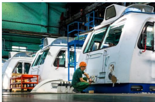
Picture 2 – Preparation of new control cabin 2 (3) ES5K for installation
