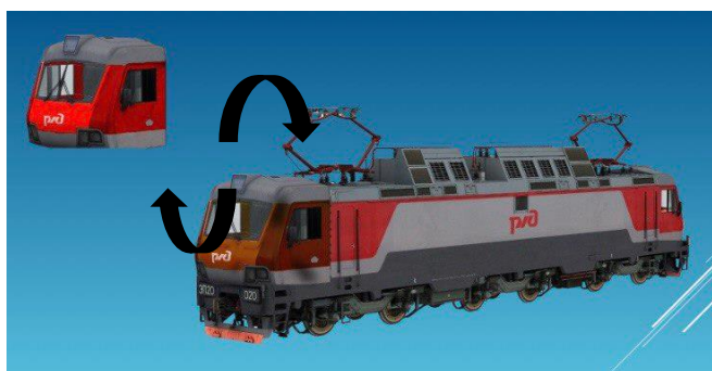
Picture 3 – Modular replacement of the control cabin
